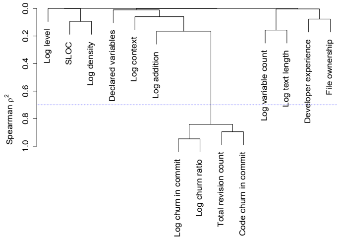
Fig. 9: Hierarchical clustering of variables according to Spearman's \rho^2 in ActiveMQ (the blue dotted line indicates our cutoff value ( |\rho^2| = 0.7 ))
